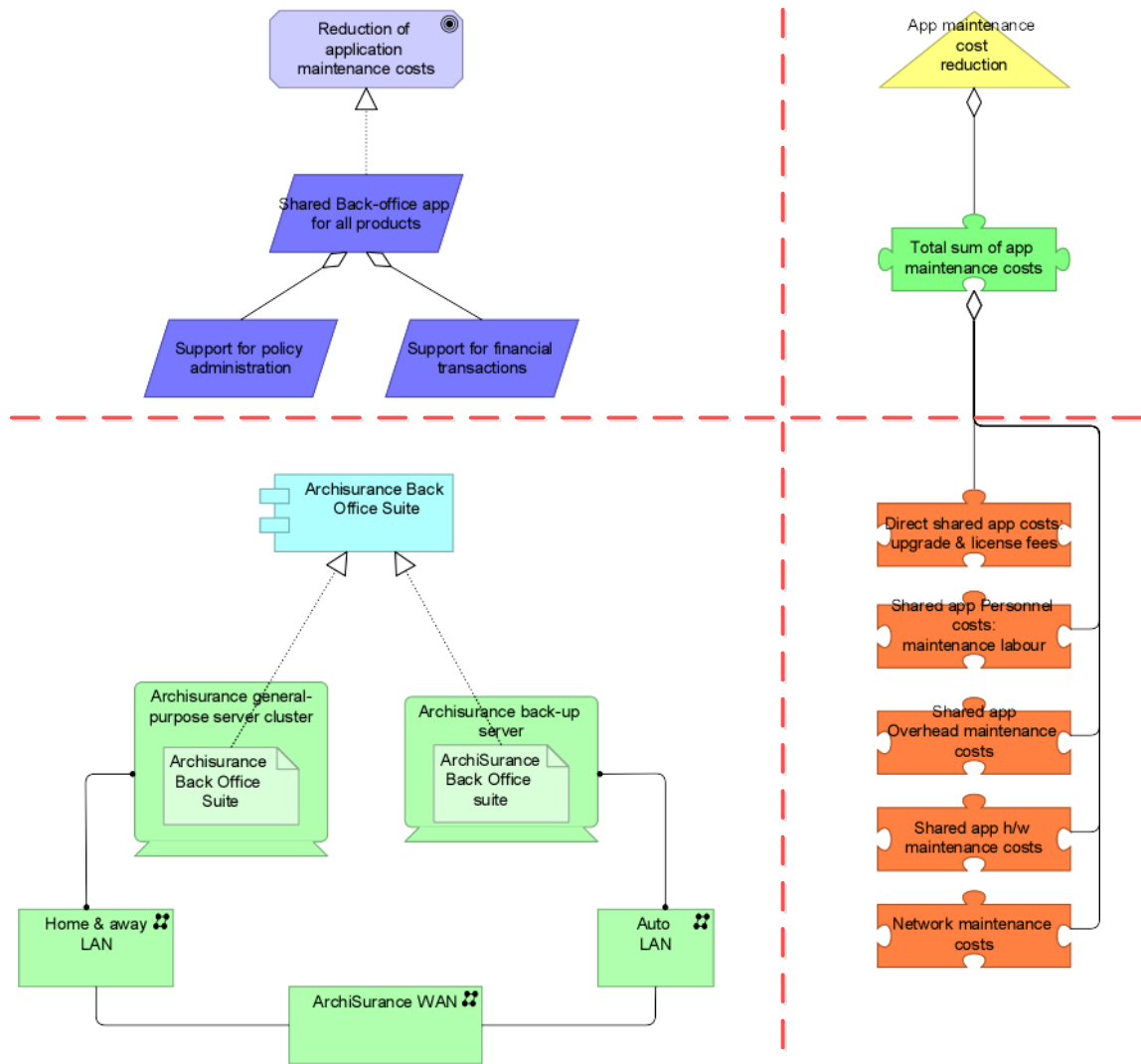
Figure 99 - Analysis model and PI structure for measuring the Shared app maintenance costs in Target EA
